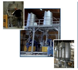
The installation is prepared to produce several t/h of finish product, working with two conveying lines installed in parallel. The products are sucked from different feeders, in function of the production order given by the supervision software. The powders are then dispensed into the final receiver.
